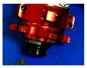
• Upgraded rear wheels can also be identified by the locknut on the non-drive side of the hub. The new locknut features the word "TIGHTEN". New "TIGHTEN" locknut = upgraded hub.
